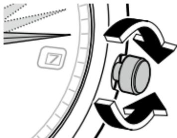
Move the minute hand ahead of the correct time by 5 "minutes" and then return the hand to the correct "minutes". This will minimize the effect of gear play and will provide more accurate hand movement.
