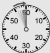
Pull out the crown just as the second hand is at the reference position in order to accurately align to the second.
