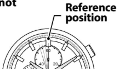
Time is stopped while aligning with the reference position. Set the time after aligning.
