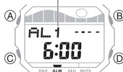
3. Press (A) to turn off the displayed alarm or the hourly time signal.
