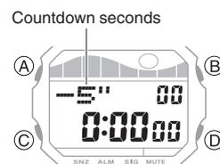
3. Press (D) to start an Auto Start operation. A countdown will begin five seconds before the start of timing. Three seconds before the start of timing, the watch will beep at one-second intervals.
