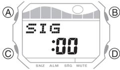
3. Press (A) to toggle the hourly time signal between enabled and disabled.
